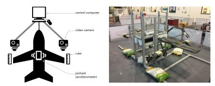
**Figure 24.** (Left) Hardware in the loop schematic for testing to the performance of a large UAV; (right) the plane is fixed to a rigid stand and through control injections, exercises the same activities as would occur during flight. Courtesy of Gilmour Space Technologies.
