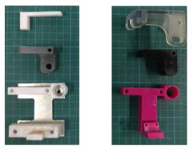
**Figure 27.** (Left) Early prototype for 3D printer extruder head, using mixture of CNC aluminum parts and 3D printed parts; (right) later prototype of the same extruder head made with fewer parts, via leveraging AM principles. Additive manufacturing, and CAD allow for the integration of parts among other strategies to reduce design effort (Perez *et al.* 2015).
