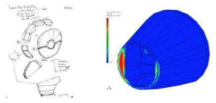
**Figure 3.** A sketch of a tiled surface, or tectonic structure to produce a re-entry capsule shell. The sketch on the left is a concept of the shell tiling, it is not a prototype as it is not tied to a test. The prototype on the right allows for testing, as it includes simulated stress loading, in a finite element model (FEM).
