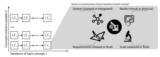
**Figure 5.** A map of the prototyping strategy space. Where  $I_iC_n$  is the *i*th iteration of the *n*th concept. Note that each block represents a single prototype or build. The expanded grey area depicts that each build has several factors of construction. The number of iterations of each concept may vary. For systems, this process can be applied at the system, subsystem, and component level.
