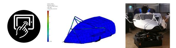
**Figure 18.** (Left) Stress loading in a finite element model (FEM) of a reusable launch vehicle (RLV) simulator; (right) Final, complete functional prototype of an RLV simulator. Courtesy of Gilmour Space Technologies.
