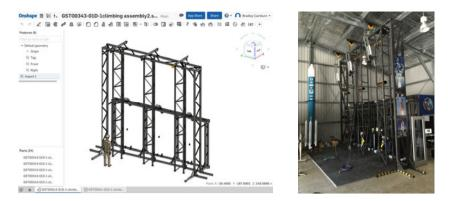
**Figure 19.** Leveraging distributed design. (Left) Engineers from Singapore and Australia co-created the CAD for this zero-gravity wall climb simulator using a web-based platform that allows for multiple users to access one file simultaneously using the Onshape software; (right) final functional design of the wall climb. Courtesy of Gilmour Space Technologies.
