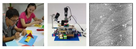
**Figure 11.** (Left) Paper mockups of the structure of an atomic force microscope casing; (center) intermediate functional prototype; (right) sample scanned image from a later prototype. In this particular design context, mockup prototyping permitted high-level assessment of many potential frame designs in parallel (with limited resources). More than thirty mockups, similar to the design in the left frame, were fabricated with paper and clay in less than 45 minutes.
