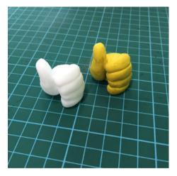
**Figure 4.** Demonstrating the replication of a handmade object using a 3D scanner to capture the design as a point cloud, which is converted to a sterolithography (STL) file and then reproduced with a fused deposition modeling (FDM) printer.
