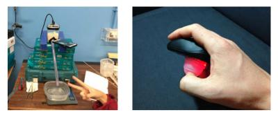
**Figure 26.** (Left) A simple configuration to test viscosity of a composite slurry using recycled storage container as a pressure vessel; (right) using rolling applicator as a modification to prototype a table-less mouse.
