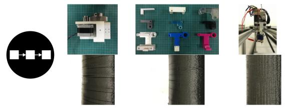
**Figure 6.** An example of iterative design. (Left) Initial design; (centre) a series of three iterative refinements; (right) the final design for a large-scale 3D printer extrusion head. The reliability of the print process gradually increased with each iteration (test prints shown below each design). The final design required nearly 40 iterations to achieve reliable printing. Courtesy of Gilmour Space Technologies.
