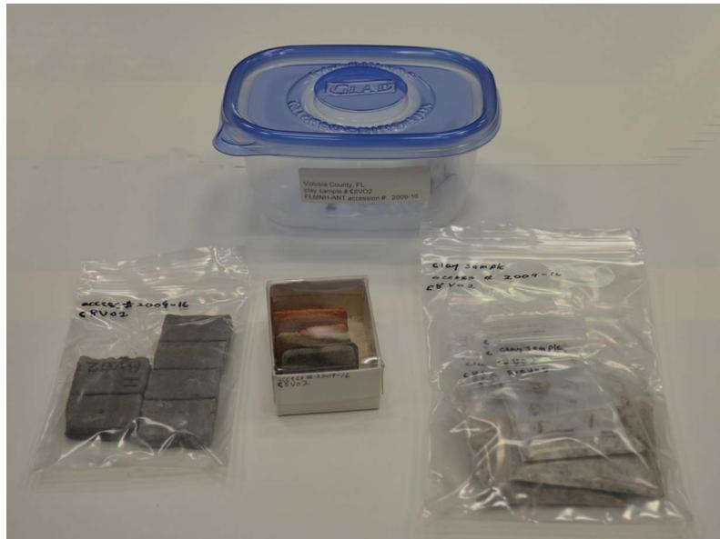
**FIGURE 13.** Processed sample clay ready for curation: (top) storage container, (bottom, left to right) leftover test bar, boxed fired briquettes, and bagged sieved sediments.
