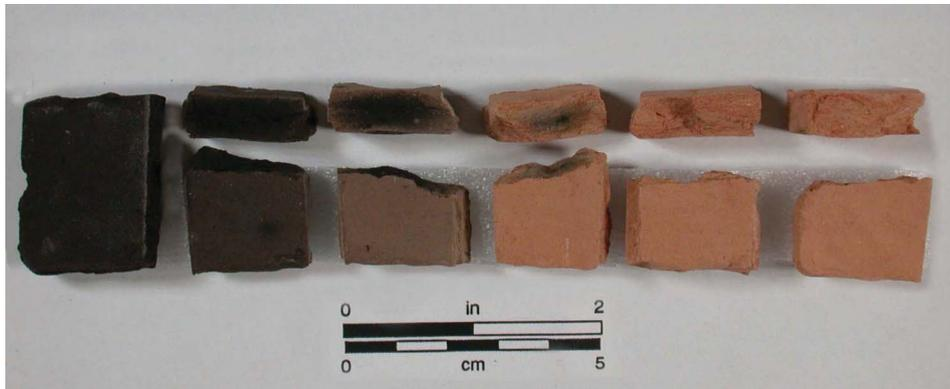
FIGURE 8. Fired briquettes are broken to record color change and coring loss.
