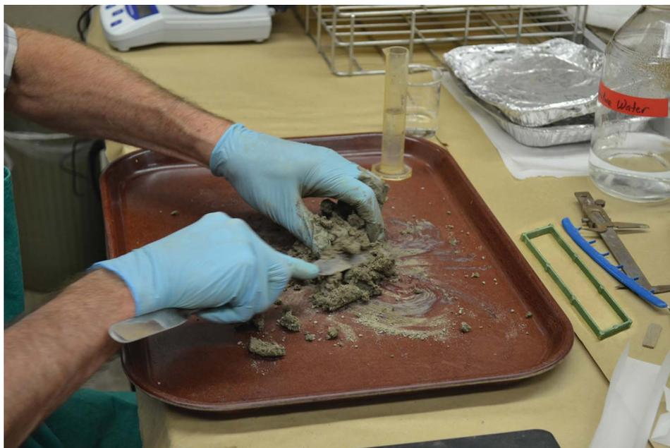
**FIGURE 2.** Working the clay and water into a plastic mass (test bar template also pictured).
