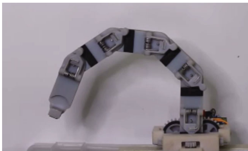
Fig. 17. By rotating the four links counter clockwise, the robot gets a C shape.
