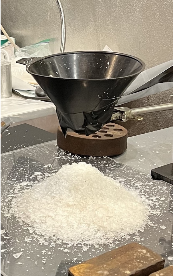
Figure 1. Image depicting the experimental setup and showing a pile formed from a mixture of 8–16 mm particles of ice +0.1 volume percent wood ash.
