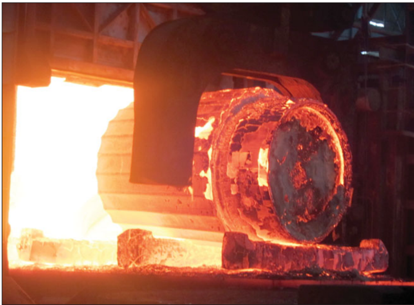
The 100-ton cast steel ingot (30Cr 2 Ni 4 Mo). Channel segregation was eliminated through purifying technology to get low oxygen content. The type of steel shown here is used for the manufacture of low-pressure rotors in nuclear power plants. Credit: Professor Dianzhong Li.
