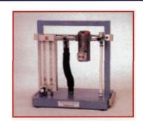
Anaesthesia Machine MP-2 This is a MP-1 with flowmeters for  $O_2$  and  $N_2O$ , as well as an  $O_2$  flush value added. The MP-2 works on the same principles as anaesthesia machines found in most hospitals. It can be used as a "Draw-over" machine if the oxygen supply fails.
