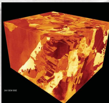
Austenitic-ferritic duplex steel, 16 x 12 x 18  $\mu\text{m}^3$  volume acquired with the AutoSlice and View™ application. A series of top-down high energy, high angle SEM-BSE images were collected automatically. The distance between each slice is 30 nm. *Courtesy of FEI NanoPort.*
