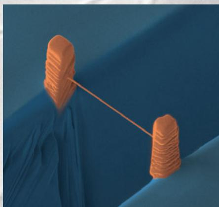
Platinum nanowire deposited and milled to about 50 nm diameter for use as a gas sensor
