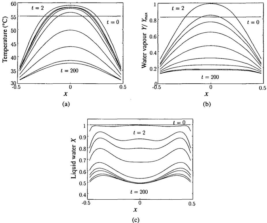
FIGURE 3. Spatial profiles of (a) temperature, (b) scaled water vapour  $Y/Y_{\max}$  and (c) liquid water  $X$  for the spatial coordinate  $x \in [-0.5, 0.5]$ .
