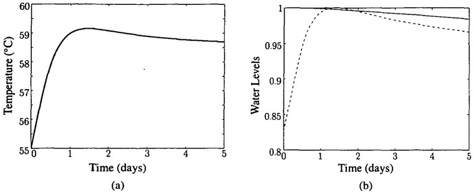
FIGURE 2. The time variation of (a) temperature and (b) liquid water  $X$  (—) and scaled water vapour  $Y/Y_{\max}$  (- - -) levels at the centre of a bagasse pile of thickness  $w = 2.2$  m.
