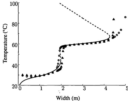
FIGURE 7. Bifurcation curve of the pile centre temperature as a function of the width  $w$  from the approximate equations is compared with the numerical results from the full system at time 30 days (o) and at 90 days ( $\Delta$ ).
