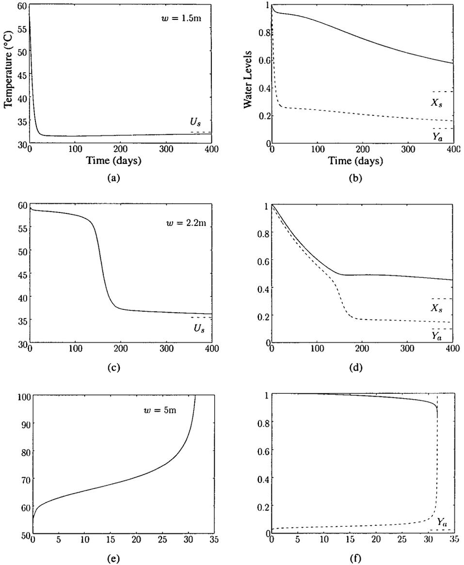
FIGURE 1. The time variation of temperature (a), (c), (e) and liquid water levels  $X$  (—) and scaled vapour  $Y/Y_{\max}$  (- - -) (b), (d) (f), at the centre of a bagasse pile of thickness  $w = 1.5, 2.2$  and  $5\text{ m}$  respectively. Steady-state values are indicated on each figure by a dot-dash line.
