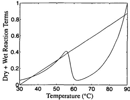
FIGURE 4. The heat release mechanism described by the dry reaction plus wet reaction and the bulk heat loss term shown as a function of temperature scaled by the value at 90° C.
