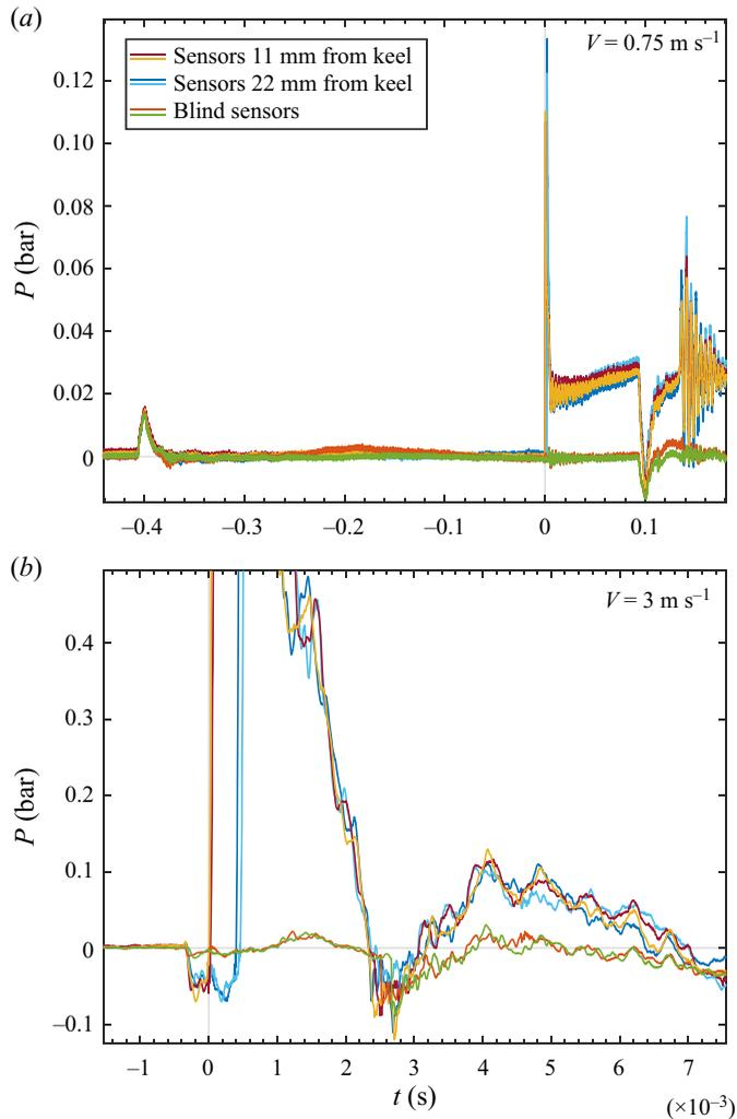
Figure 15. (a) Pressure measurements from all sensors at  $V = 0.75 \text{ m s}^{-1}$  and (b) at  $V = 3 \text{ m s}^{-1}$ . In (a) we show both the start and end of the impactor’s motion. In (b) we only show the region closer to impact to show the differences between the exposed and blind sensors. The plot legend is shared between panels (a) and (b).
