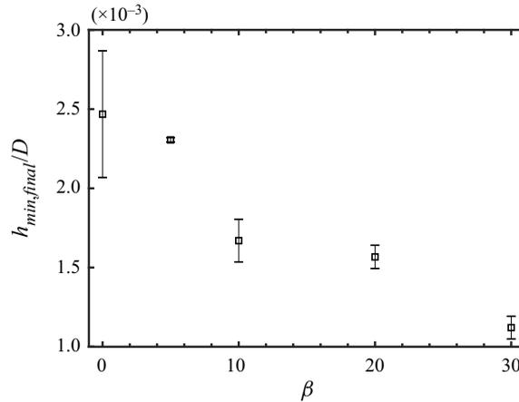
Figure 13. The non-dimensionalised final depth  $h_{min,final}$  of the surface deformation due to air cushioning is plotted vs the deadrise angle for a disc and several cones with diameter  $D = 70$  mm and impact speeds  $V$  varying between  $0.7$  and  $3.5$  m s<sup>-1</sup>. The error bars denote the variation occurring for different impact speeds.
