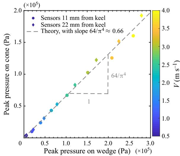
Figure 8. The peak pressures from wedge and cone are directly compared at both sensors. The peak pressures measured on the cone are found to be  $64/\pi^4$  times to those measured on the wedge across the whole range of  $V$  used. The measurements are compared with the analytical result (2.25) finding excellent agreement.
