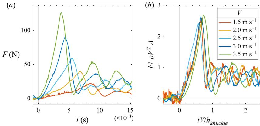
Figure 16. (a) Time series of the force  $F$  during impact of a cone with a deadrise angle of  $30^\circ$ , measured for five different impact velocities. (b) The same data as in (a) but now non-dimensionalised with inertial force ( $\rho V^2 A$ ) and time ( $h_{knuckle}/V$ ) scales, leading to a fair collapse of the data.
