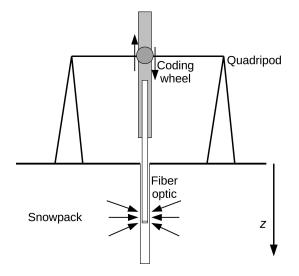
Fig. 3. Schematic illustration of the irradiance profiler SOLEXS.
