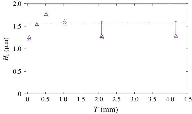
FIGURE 5. Plot of the first maximum of the centreline height of the air disc  $H^*$  versus the liquid film thickness,  $T$ , for impacts of  $10^4$  cSt silicone oil drops onto liquid films of the same liquid with  $R_b = 1.4$  mm and  $V = 1.4$  m  $\text{s}^{-1}$ .
