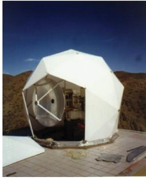
**Figure 8.** The Solar Submillimeter Telescope, a solar dedicated radio antenna installed in Argentina operating at 212 and 405 GHz.
