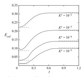
Figure 10. Numerical results for the transient collision efficiency with respect to time for Eg = 0,  $a_p = 0.5$  and different values of non-dimensional permeability:  $K^* = 10^{-2}$ ,  $K^* = 10^{-3}$ ,  $K^* = 10^{-4}$  and  $K^* = 10^{-5}$ . The dashed lines represent the theoretical results for the initial and steady-state collision efficiencies.
