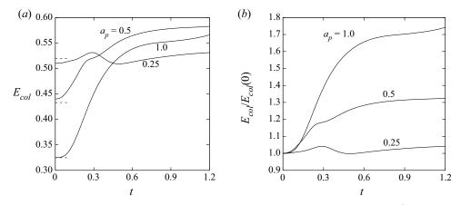
Figure 12. Numerical results for the transient collision efficiency for Eg = 0.25,  $K^* = 10^{-4}$  and different values of particle radii:  $a_p = 0.25$ ,  $a_p = 0.5$  and  $a_p = 1.0$ . Here, (a) shows the values for the transient collision efficient, whereas, in (b), the results are normalized by the numerical value for the initial collision efficiency. The dashed lines represent the theoretical results for the initial and steady-state collision efficiencies.
