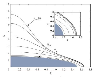
Figure 6. Collision boundaries for Eg = 1.0,  $K^* = 10^{-4}$ ,  $a_p = 0.5$ , and (in to out) t = 0.02, 0.1, 0.3, 0.5, 0.7, 0.9 and 1.0. The inset shows a zoom of the details of the right region of the graph, where the curves start to coincide. The shaded region represents the inside of the collision surface  $r = 1 + a_p$ . The collision volume  $(V_{col})$  is the unshaded region between the collision surface  $(S_{col})$  and the collision boundary  $(A_{col})$ .
