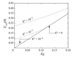
Figure 4. Initial collision efficiency versus the engulfment parameter for  $a_p = 0.5$  and different values of non-dimensional permeability. The solid line represents the limit where  $K^* \rightarrow 0$ , and, hence,  $(1 - A_0) = 0$ .
