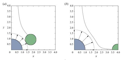
Figure 2. Trajectory simulation for Eg = 1.0,  $K^* = 10^{-4}$ ,  $a_p = 0.5$  and  $z_0 = 4.0$ , with (a)  $x_0 = 0.6$  and (b)  $x_0 = 0.7$ . The dashed line represents the final interface of the drop at the end of the trajectory. In (a), the solid particle is captured by the expanding drop, whereas the trajectory in (b) does not result in aggregation.
