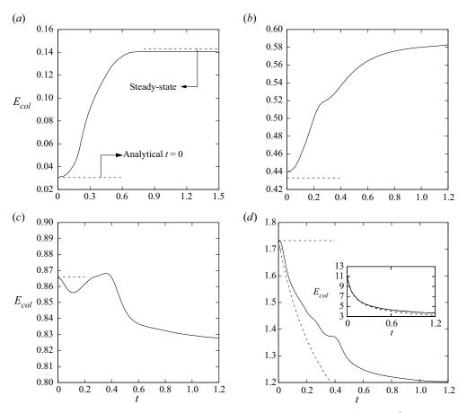
Figure 9. Numerical results for the transient collision efficiency versus time for  $K^* = 10^{-4}$ ,  $a_p = 0.5$  and engulfment parameters (a) Eg = 0, (b) Eg = 0.25, (c) Eg = 0.5, (d) Eg = 1.0 and 7.0 (in inset). The dashed lines represent the analytical solution at t = 0, and the value of the theoretical steady-state collision efficiency in (a). The dashed curve in (d) is the pure expansion collision efficiency, as described by (3.9) and (3.22).
