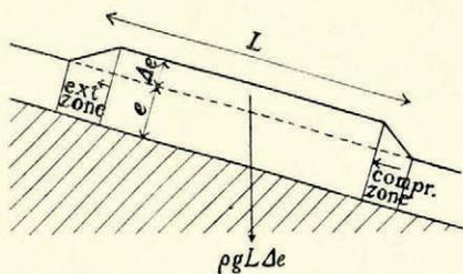
Fig. 3 (left). Schematic bulge going down a glacier
