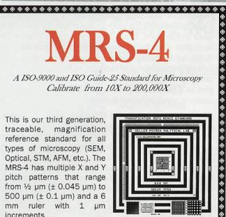
A ISO-9000 and ISO Guide-25 Standard for Microscopy Calibrate from 10X to 200,000X
