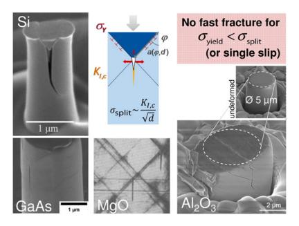
Figure 5. Axial splitting and suppression of fast fracture in semiconductors and oxide ceramics. Splitting model/geometry from Ref. 2 Reprinted with permission by Taylor & Francis Ltd. (www.tandfonline.com) from Ref. 2, John Wiley and Sons from Ref. 1 and Springer from Ref. 97, (Al<sub>2</sub>O<sub>3</sub>: unpublished).
