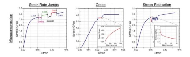
Figure 9. Studies of rate sensitivity in nickel, including rate jump testing, creep, and relaxation hold segments in microcompression inside the SEM.<sup>[38]</sup> Reprinted with permission by Elsevier from Ref. 38.
