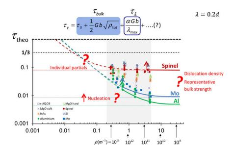
Figure 7. Comparison of the effect of size on critical resolved shear stress across material classes, including FCC AI (unpublished), BCC Mo, [98] the soft  $\{110\}\frac{1}{2}\langle \overline{1}10\rangle$ , and hard  $\{001\}\frac{1}{2}\langle \overline{1}10\rangle$  slip systems in MgO, [70] the oxide ceramics MgAl<sub>2</sub>O<sub>4</sub> spinel, and Al<sub>2</sub>O<sub>3</sub> alumina (unpublished) as well as the semiconductors InAs (unpublished) and Si. [31]
