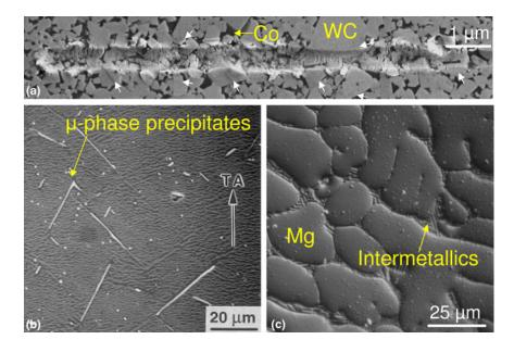
**Figure 1.** Examples of hard phases in engineering materials. (a) Tungsten carbide in the cemented carbide WC-Co exhibiting plastic deformation in nanoscratch testing, (b) topologically close-packed μ-phase precipitates in a nickel-based superalloy after creep-testing and (c) intermetallic skeleton included in cast Mg–Al–Ca alloy to increase creep resistance. [images: (a) courtesy of J. S. K.-L. Gibson; (b) Reprinted with permission from Elsevier Ref. 86; (c) courtesy of C. Zehnder].
