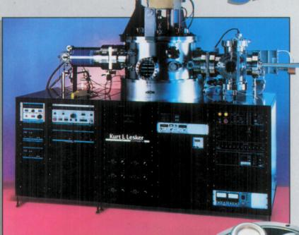
Supersystem III four-station, sputter-up deposition system.
