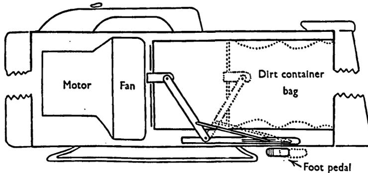
Fig. 1. Hoover 402. Diagram of emptying mechanism.
