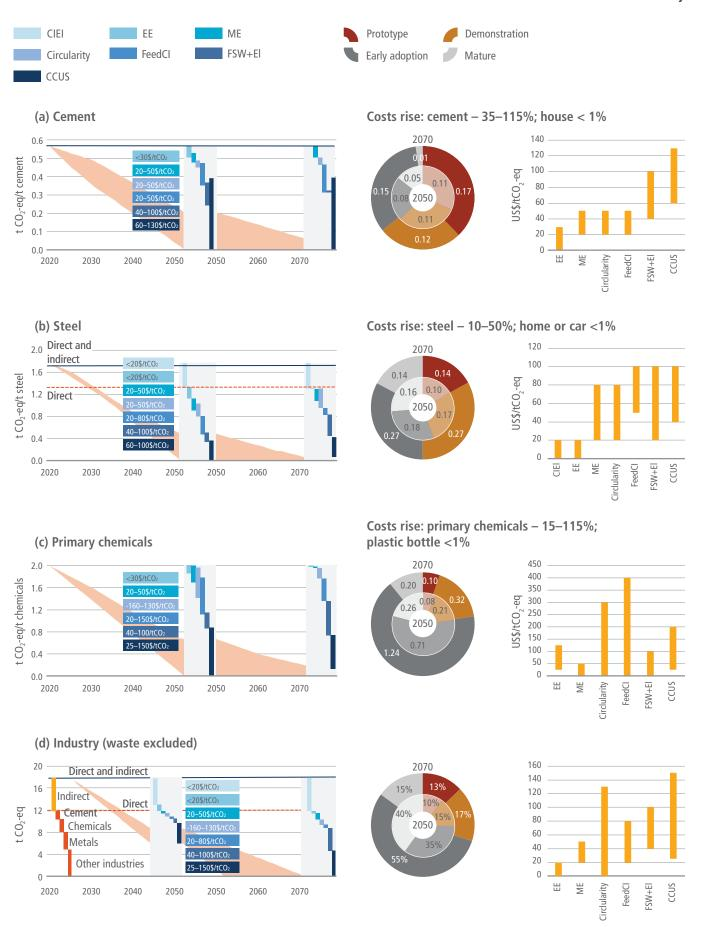
Figure TS.17 | Potentials and costs for zero-carbon mitigation options for industry and basic materials.
