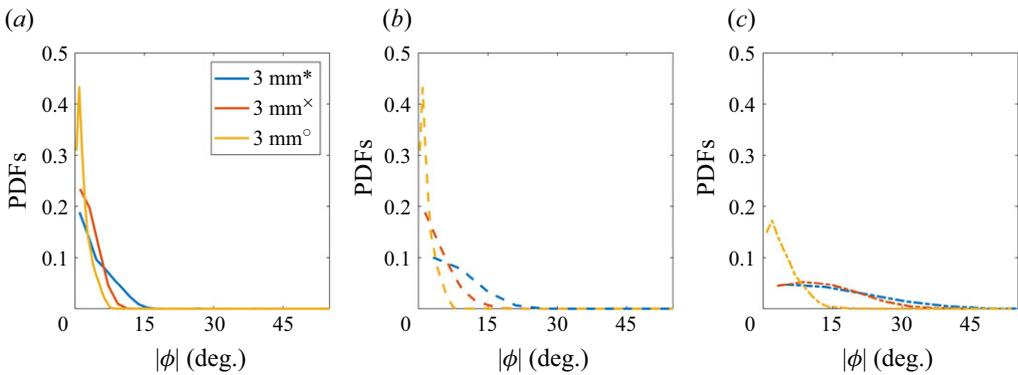
Figure 9. Distributions of two-dimensional projected trajectory angles off the vertical,  $|\phi|$ , plotted for each disk type in (a) quiescent air, (b) weaker turbulence and (c) stronger turbulence. Colours correspond to those assigned by disk type as in figure 8.
