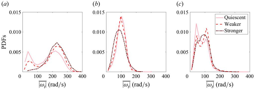
Figure 11. Trajectory-averaged angular velocity distributions for all flow conditions for the (a) 3 mm\*, (b) 3 mm<sup>x</sup> and (c) 3 mm<sup>o</sup> disks.
