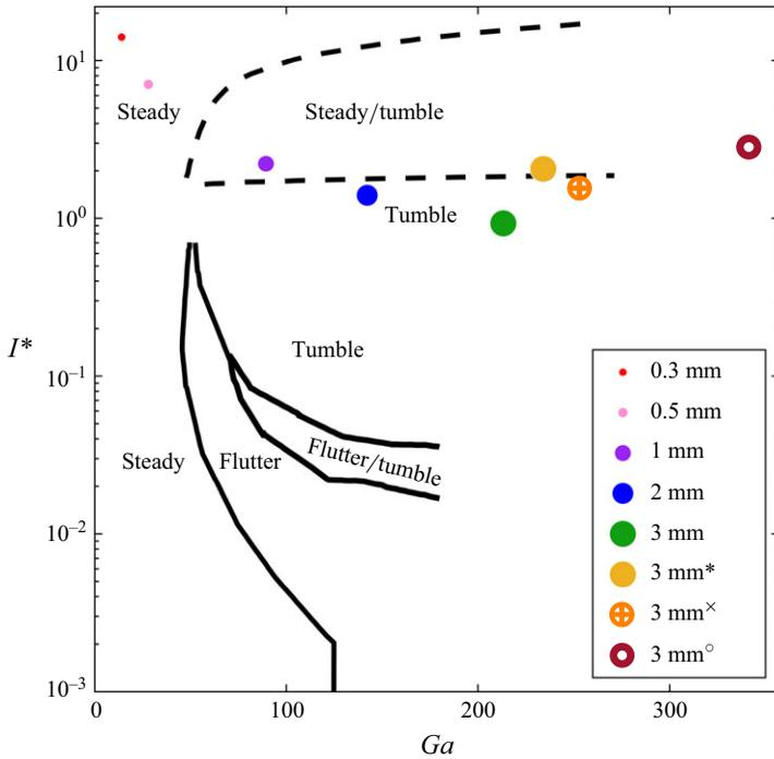
Figure 4. Falling style parameter space of  $I^*$  versus  $Ga$  with disks in the current study placed among data from the literature. Solid black lines show the falling mode boundaries identified by Auguste *et al.* (2013). Dashed black lines indicate upper and lower boundaries of the region of bistability found by Lau *et al.* (2018).
