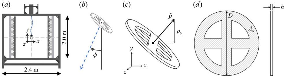
Figure 3. (a) Turbulence facility diagram including global coordinate system and basic dimensions. (b) Definition of the disk trajectory angle  $\phi$ . (c) Representation of the disk orientation vector  $\hat{p}$  and its vertical component  $p_y$ . (d) Definition of the disk solid area  $A_s$ , nominal diameter  $D$ , and thickness  $h$ .
