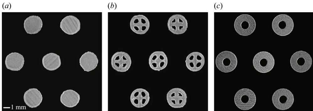
Figure 2. Image groupings of laser cut and perforated disks showing the variation within the populations of the (a) 3 mm\*, (b) 3 mm<sup>×</sup> and (c) 3 mm<sup>°</sup>.
