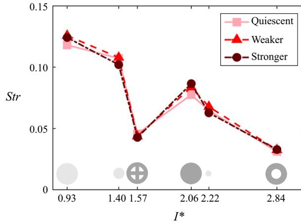
Figure 13. Strouhal number  $Str$  plotted as a function of  $I^*$ , with respective disk geometry shown along the abscissa. Light coloured disks represent those with  $h = 50 \mu\text{m}$  and darker represent  $h \approx 100 \mu\text{m}$ .
