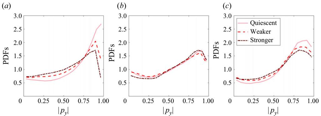
Figure 7. The PDFs of the modulus of the instantaneous disk orientation vector with respect to the vertical,  $|p_y|$ . Plotted at each forcing level for the (a)  $3\text{ mm}^*$ , (b)  $3\text{ mm}^\times$  and (c)  $3\text{ mm}^\circ$  disks. Here,  $|p_y| \sim 0$  indicates an edge-on orientation and  $|p_y| \sim 1$  indicates a flat-falling orientation.
