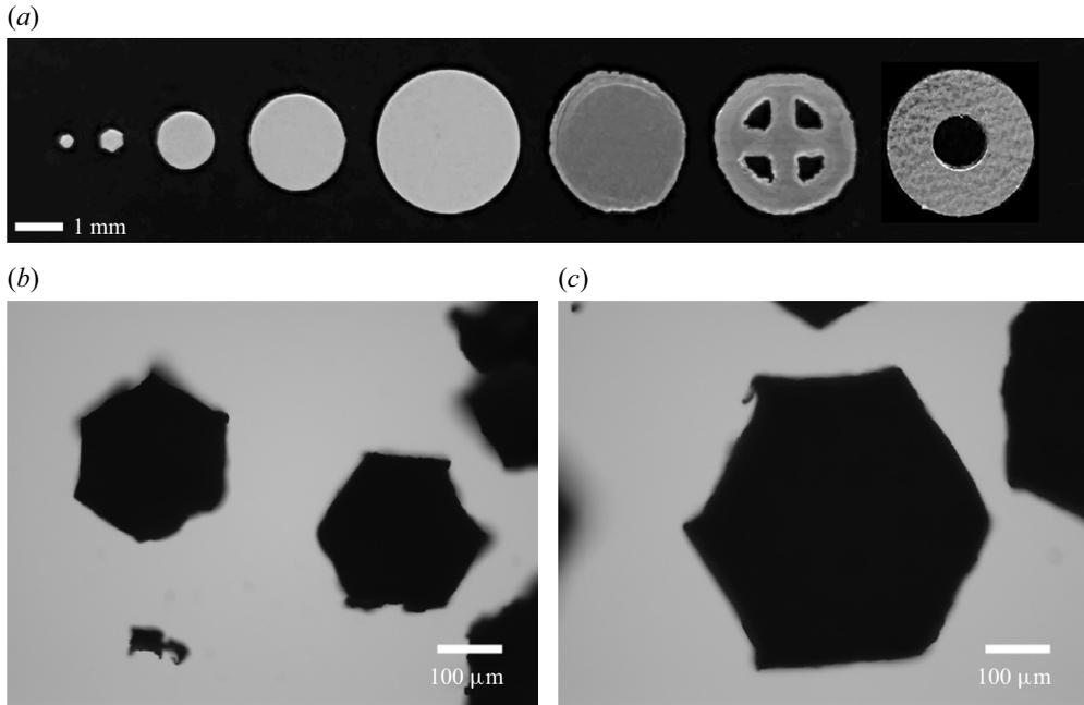
Figure 1. Images of all disks studied. (a) From left to right,  $D$  increasing from 0.3 to 3 mm $^\circ$ . (b) Microscope images of 0.3 mm and of (c) 0.5 mm disks.
