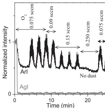
**Figure 4.** Time resolved OES following the impact of oxygen flow on dust formation.
