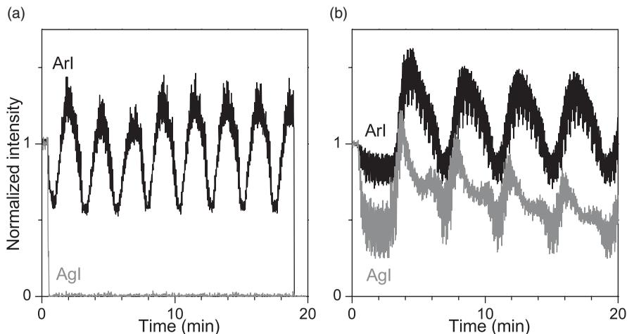
**Figure 1.** Time-resolved OES of argon (549.6 nm) and silver (546.5 nm) lines. Dust synthesis (a) without silver sputtering ( $P=10$  W, HMDSO average flow = 0.28 sccm), and (b) with silver sputtering ( $P=30$ W, HMDSO average flow = 0.12 sccm).
