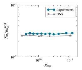
FIGURE 2. (Colour online) Compensated form of the dependence of Nusselt number  $\overline{Nu}$  on the Rayleigh number  $Ra_H$  for the single-phase case.
