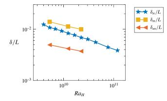
FIGURE 10. (Colour online) Normalised boundary layer thickness in the single-phase case as a function of  $Ra_H$ . Here  $\delta_{un}$  and  $\delta_{tn}$  are numerically obtained thickness of the kinetic and thermal boundary layer, respectively. The thickness of the thermal boundary layer obtained from the experiments is given as  $\delta_{te}$ .
