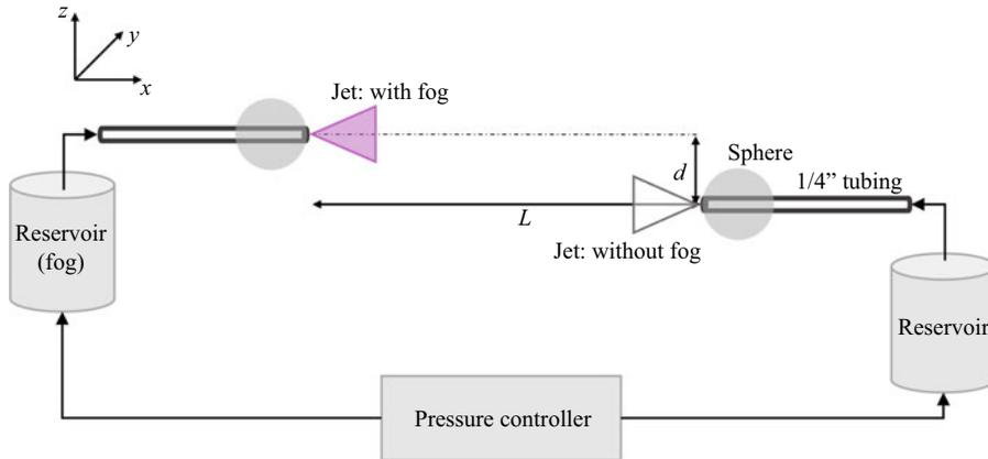
Figure 2. Experimental set-up. Two spheres are placed an axial distance  $L$  apart with a transverse offset  $d$ . A reservoir supplies pressurized air, set by a pressure controller, to the tubing, which goes through the hollow sphere. One reservoir is seeded with fog for visualization of the jet using a laser sheet in the  $xz$ -plane.
