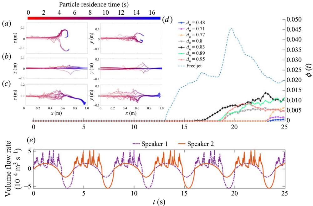
Figure 6. Side and top views of the trajectory of particles with highest streamwise reach for  $L = 1$  m: (a)  $d_n = 0$ , (b) free jet, and (c)  $d_n = 0.83$  (movie 6). (d) Graph showing  $\phi(t) \equiv N_H/N_i$  for different offsets. (e) Volume flow-rate signals for speaker 1 (violet) and 2 (orange).
