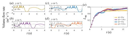
Figure 5. The effect of phase lag on the streamwise propagation of the particle cloud. (a-d) The dotted line represents the volume flow-rate signal of speaker 1 and the solid coloured lines are for speaker 2 with the phase lag  $\psi$  as indicated in the panels. (e) The streamwise length ( $L_{90}$ ) versus time for phrase 'S' is shown for phase lags  $\psi = 0-5.2$  s.
