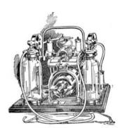
The outstanding feature of this apparatus is that there are two separate pairs of cylinders for pressure and for suction, without intercommunication between them; so the pressure cylinders cannot possibly become contaminated by anything that has been drawn away from any patient.
