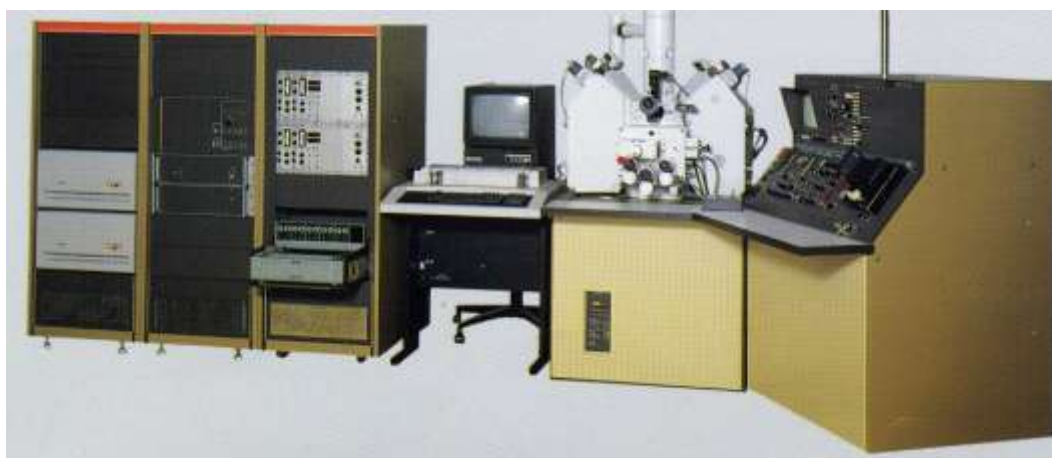
FIG. 1: Original Jeol 733 Probe that consumed 8KVA power in full operation. Image courtesy of Jeol.
