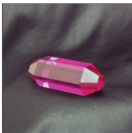
Figure 2. Ruby laser crystal prepared for the MRS Von Hippel Award trophy. Length, ~5 cm. Photo by Kristin Wilson.
