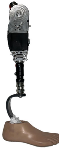
Figure 1. Image of the Vanderbilt powered knee prosthesis used in this work.
