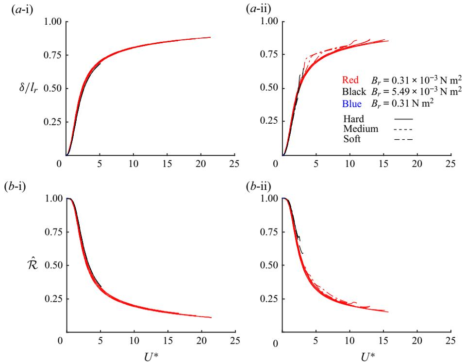
Figure 12. Theoretical predictions of (a) dimensionless tip deflection  $\delta/l_r$  and (b) reconfiguration number  $\hat{\mathcal{R}}$  in a broad range of  $U^*$ :  $B_r = 0.31 \times 10^{-3} \text{ N m}^2$  (red),  $5.49 \times 10^{-3} \text{ N m}^2$  (black), and  $0.31 \text{ N m}^2$  (blue). Here, (i) and (ii) are for the power and recovery strokes, respectively.
