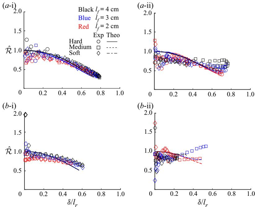
Figure 20. New reconfiguration number  $\hat{\mathcal{R}}$  for (a) cases with a thin centre rod, and (b) cases with a thick centre rod with respect to dimensionless tip deflection magnitude  $\delta/l_r$ , where (i) and (ii) are for the power and recovery strokes, respectively. Symbols and lines denote experimental and theoretical results, respectively.
