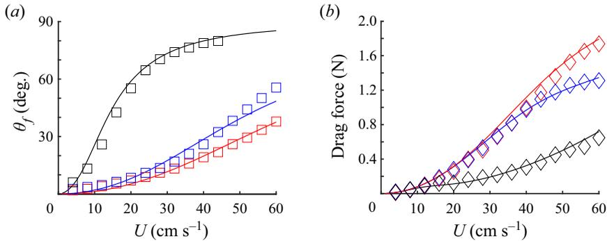
Figure 4. (a) Hinge angle  $\theta_f$  obtained from experiment ( $\square$ ) and theoretical prediction using (3.1) (solid lines). (b) Drag force obtained from force transducer measurement ( $\diamond$ ) and theoretical prediction using (3.1) and (3.2) (solid lines). Red, blue and black correspond to hard, medium and soft hinges, respectively. Straight centre rods with  $\theta_r = 0$  are used to neglect the effect of centre-rod deflection on the folding of the side flaps.
