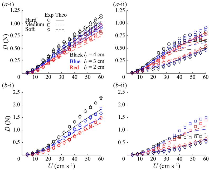
Figure 19. Dimensional quasi-steady drag force  $D$  with respect to dimensional speed  $U$  for (a) cases with a thin centre rod, and (b) cases with a thick centre rod, where (i) and (ii) are for the power and recovery strokes, respectively. Symbols and lines denote experimental and theoretical results, respectively.
