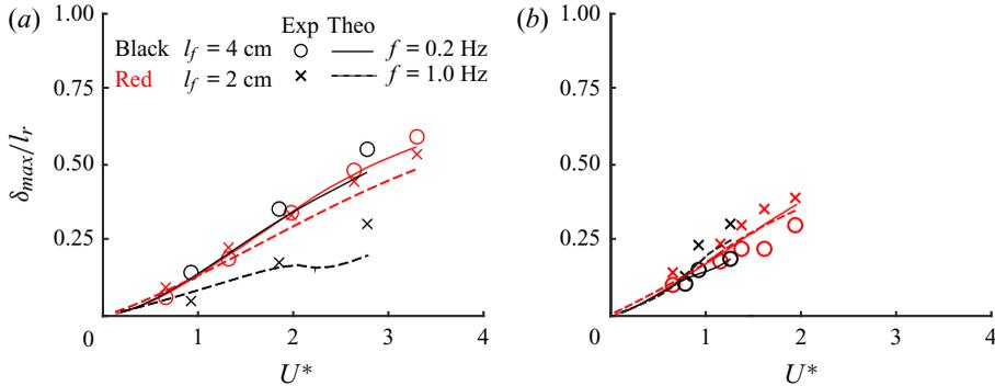
Figure 16. Maximum magnitude of tip deflection  $\delta_{max}/l_r$  during (a) the power stroke and (b) the recovery stroke, for  $l_f = 2$  and 4 cm (s2 and s4 in table 2). Symbols and lines denote experimental and theoretical results, respectively.
