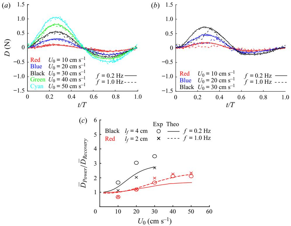
Figure 17. Time histories of dimensional drag force  $D$  acting on the elastic structure over a single cycle for (a)  $l_f = 2$  cm and (b)  $l_f = 4$  cm. (c) Ratio of time-averaged drag forces between power and recovery strokes,  $\bar{D}_{Power}/\bar{D}_{Recovery}$ , versus dimensional speed amplitude  $U_0$ . In (c), symbols and lines denote experimental and theoretical results, respectively.
