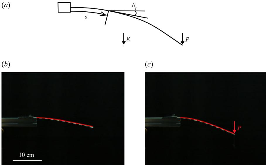
Figure 2. (a) Schematic of the elastic structure under gravity and with a point load  $P$  at the free end. (b,c) Raw images of the bent elastic structure and theoretically estimated profiles (red solid lines) using (2.1): (b) under gravity only; (c) under gravity with the point load at the free end.
