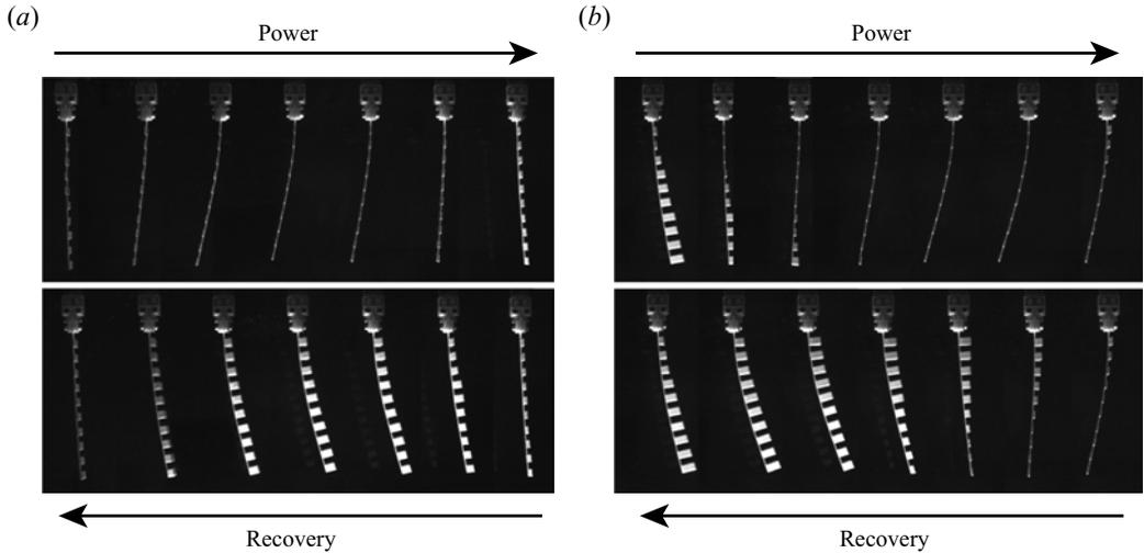
Figure 14. Sequential images of the oscillating elastic structure over a single cycle for  $l_f = 2$  cm ( $s$  in table 2) with speed amplitude  $U_0 = 20$  cm s<sup>-1</sup>, and oscillation frequencies (a)  $f = 0.2$  Hz and (b)  $f = 1.0$  Hz.
