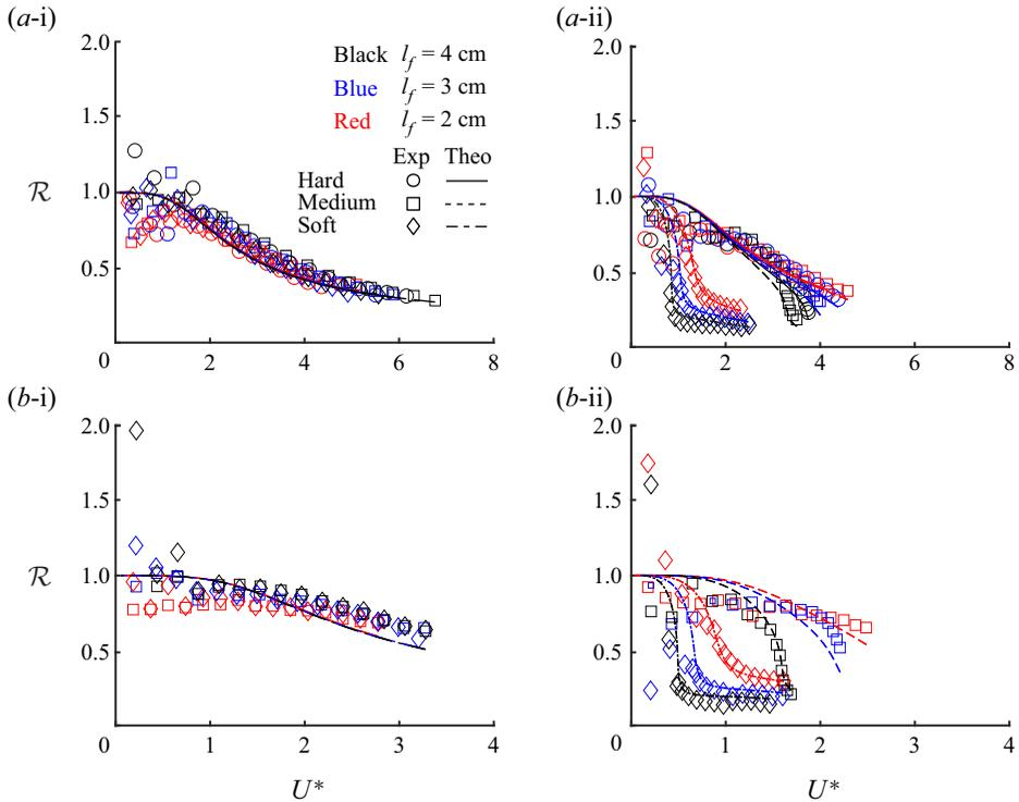
Figure 9. Reconfiguration number  $\mathcal{R}$  for (a) cases with a thin centre rod (small letters in table 2), and (b) cases with a thick centre rod (capital letters in table 2), where (i) and (ii) are for the power and recovery strokes, respectively. Symbols and lines denote experimental and theoretical results, respectively.
