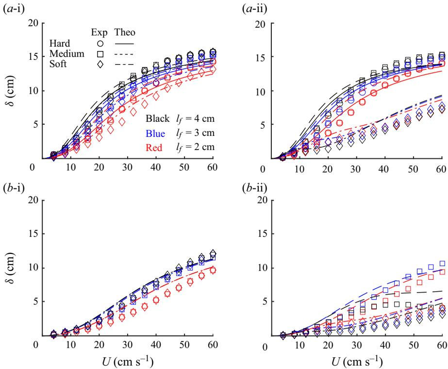
Figure 18. Dimensional amplitude of tip deflection  $\delta$  with respect to dimensional speed  $U_0$  for (a) cases with a thin centre rod, and (b) cases with a thick centre rod, where (i) and (ii) are for the power and recovery strokes, respectively. Symbols and lines denote experimental and theoretical results, respectively.
