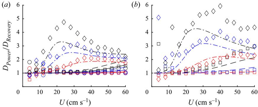
Figure 11. Force ratio between power and recovery strokes,  $D_{Power}/D_{Recovery}$ , versus dimensional translational speed  $U$  for cases with (a) a thin centre rod, and (b) a thick centre rod. Symbols and lines are from experimental and theoretical results, respectively. Symbols, line types and colours denote the same parameters as in figures 8 and 10.
