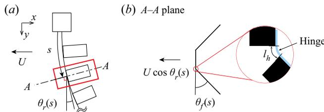
Figure 3. (a) Side view of the elastic structure during the recovery stroke in the  $(x, y)$  plane. (b) Cross-sectional view of the deflected side flaps in the  $A$ – $A$  plane marked in (a). Here,  $\theta_r$  is the deflection angle of the centre rod, and  $\theta_f$  is the deflection angle of the side flap.
