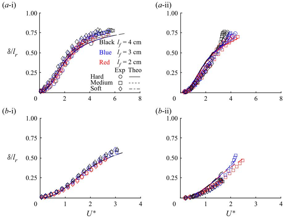
Figure 8. Amplitude of tip deflection  $\delta/l_r$  for (a) cases with a thin centre rod (small letters in table 2), and (b) cases with a thick centre rod (capital letters in table 2), where (i) and (ii) are for the power and recovery strokes, respectively. Symbols and lines denote experimental and theoretical results, respectively.
