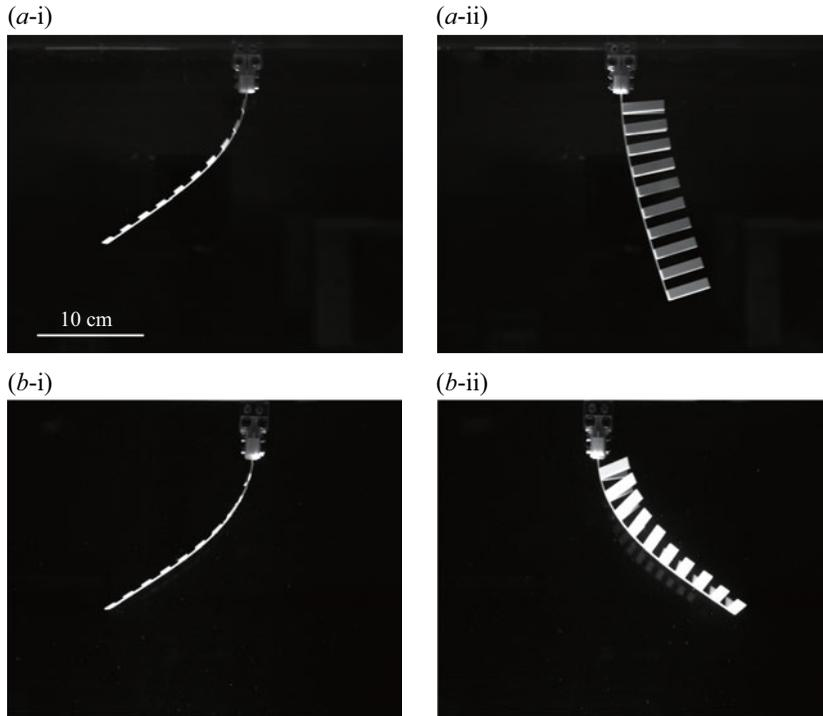
Figure 5. Raw images of the deformed elastic structure during (i) the power stroke and (ii) the recovery stroke: (a) soft-hinge case (s4), and (b) medium-hinge case (m4), in table 2. Here,  $U = 40 \text{ cm s}^{-1}$ . See the supplementary movies available at <https://doi.org/10.1017/jfm.2022.970>.
