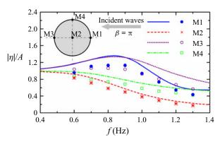
Figure 4. Deflection of four markers (M1–M4) placed on a free-floating elastic disk with R = 0.72 m, h = 1.9 m,  $\bar{\chi} = 3.55 \times 10^{-4}$  and  $\bar{\gamma} = 2.79 \times 10^{-3}$  as a function of frequency. Lines represent the present theoretical results with N = 4,  $r_0/R = 0.5$ ,  $\bar{c} = 10^{-5}$ ; symbols represent the experimental data (Montiel *et al.* 2013*b*).
