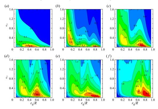
Figure 9. Contour plots for the variation of  $\eta_e$  as a function of PTO position  $r_0/R$  and PTO damping coefficient  $\bar{c}$ , for R/h = 2.0,  $\beta = \pi/6$  and kh = 4.0: (a) N = 1; (b) N = 2, (c) N = 3, (d) N = 4, (e) N = 5, and (f)  $N = \infty$ .
