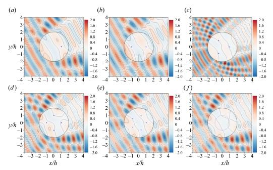
Figure 8. Deflection of the floating elastic disk,  $\text{Re}(\eta \, \text{e}^{-\text{i}\omega t})/A$ , and the near-field wave motion,  $\text{Re}(\eta_w \, \text{e}^{-\text{i}\omega t})/A$ , at t=0 for R/h=2.0,  $r_0/R=0.5$  and  $\beta=\pi/6$ : (a) N=1,  $(kh,\bar{c})=(4.28,0.04)$ ; (b) N=2,  $(kh,\bar{c})=(3.91,0.06)$ ; (c) N=3,  $(kh,\bar{c})=(7.64,0.08)$ ; (d) N=4,  $(kh,\bar{c})=(5.51,0.20)$ ; (e) N=5,  $(kh,\bar{c})=(4.65,0.12)$ ; and  $(f) N=\infty$ ,  $(kh,\bar{c})=(5.03,0.24)$ .
