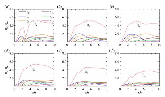
Figure 11. The partition of capture factor into contributions from different circular mode components for operation tuned to be optimal for the *m*th mode, with R/h = 2.0,  $r_0/R = 0.5$ ,  $\beta = 0$  and  $\text{Im}(\bar{c}) = 0$ : (a) m = 0, (b) m = 1, (c) m = 2, (d) m = 3, (e) m = 4, and (f) m = 5.
