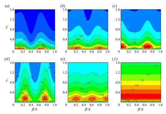
Figure 6. Contour plots for the variation of  $\eta_e$  as a function of incident wave direction  $\beta$  and PTO damping coefficient  $\bar{c}$ , for R/h=2.0,  $r_0/R=0.5$  and kh=4.0: (a) N=1, (b) N=2, (c) N=3, (d) N=4, (e) N=5, and (f)  $N=\infty$ .
