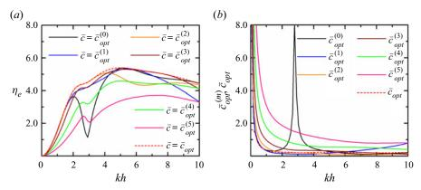
Figure 10. (a) Capture factor against dimensionless wavenumber for R/h = 2.0,  $r_0/R = 0.5$ ,  $\beta = 0$  and  $\text{Im}(\bar{c}) = 0$ , with (b) corresponding damper values optimised in order to capture the available power in the *m*th circular mode component as much as possible.
