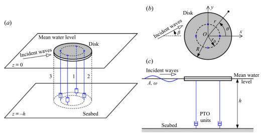
Figure 2. Sketch of a floating elastic disk-shaped WEC with a discrete PTO system (N = 4): (a) bird's-eye view, (b) top view, (c) side view.
