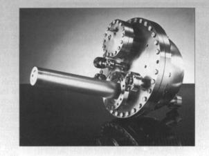
The HA54 analyser, with proven 4 element lens optics, together with the VSW range of goniometers provides state-of-the-art instrumentation for angle resolved studies.
