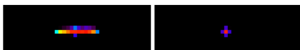
Fig. 2: The charge spilling over the pixel boundaries spreads preferentially in the direction perpendicular to the transfer. In the anti-blooming mode all charge is contained in a single pixel.
