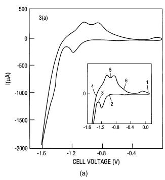
FIG. 3(a). Cyclic voltammogram for a Pd-capped multilayer 800 Å/200 Å/800 Å Nb/Pd/Nb film grown on Cr-coated float glass. The numbering from 1 to 6 corresponds to regions where  $\theta$ -2 $\theta$  scans of the Pd[111] peak were taken along the c-axis.
