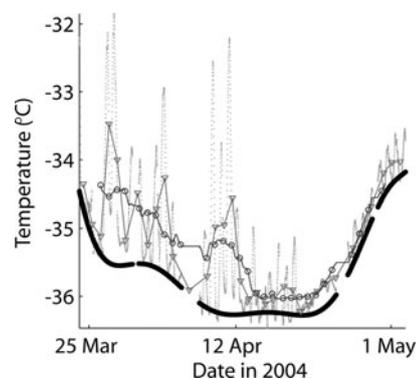
**Fig. 9.** Corrected (solid black curve) and uncorrected (light-gray dots) thermocouple data at 1.5 m depth for our Greenland dataset. Averaging the measured data over 24 hours (gray connected triangles) or applying a 5 day running mean (black connected circles) produces fictitious temperature variations with  $0.2$ – $0.5^\circ\text{C}$  amplitude and  $\sim 9$  day period.
