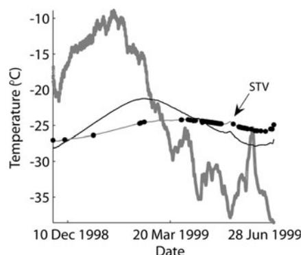
**Fig. 5.** STVs in Siple Dome data are only present in the latter half of the time series, when the reference temperature (thick gray curve) begins to decrease and show larger temporal variations. The data at 4 and 6.15 m depth are indicated by a thin black curve and thin gray curve respectively. The data used to fit the ninth-order polynomial that defines the smooth variation in temperature at 6.15 m depth are indicated by black points.
