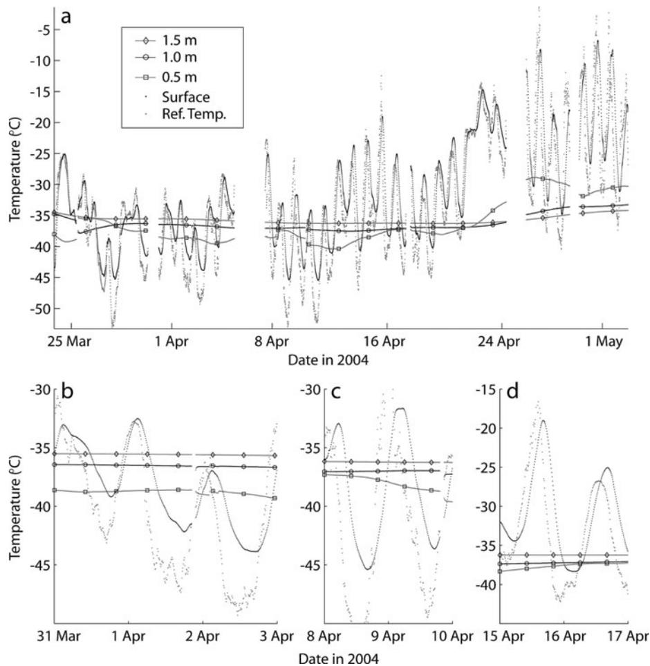
**Fig. 6.** (a) Corrected thermocouple data from the surface (gray dots), 0.5 m depth (gray curve with black squares), 1.0 m depth (black curve with black circles), 1.5 m depth (gray curve with black diamonds) and the reference temperature (black dots) within the unperturbed snowpack in Summit, Greenland, between 20 March and 30 April 2004. Cf. Figure 1.
