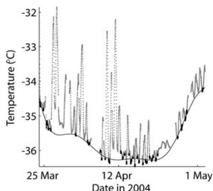
**Fig. 4.** Measured thermocouple temperatures (10 min average) at 1.5 m depth (small gray points). Measurements when the data-logger thermistor reference temperature was between  $-30$  and  $-33^{\circ}\text{C}$  are indicated by black points. The solid curve is a best-fit (ninth-order) polynomial regression through the black points.
