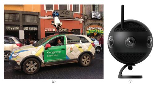
**Figure 1.9** An important component for achieving telepresence is to capture a panoramic view. (a) A car with cameras and depth sensors on top, used by Google to make Street View. (b) The Insta360 Pro 2 captures and streams omnidirectional videos.
