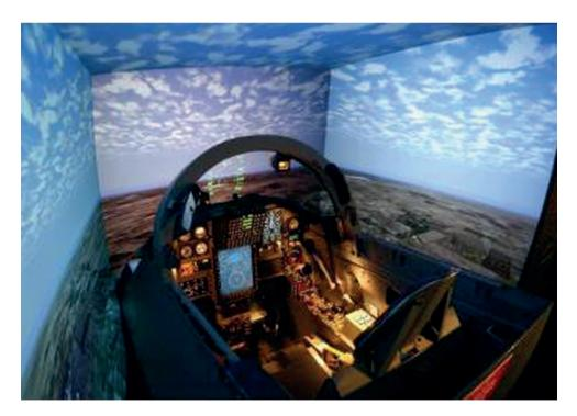
**Figure 1.16** A flight simulator in use by the US Air Force. The user sits in a physical cockpit while being surrounded by displays that show the environment.
