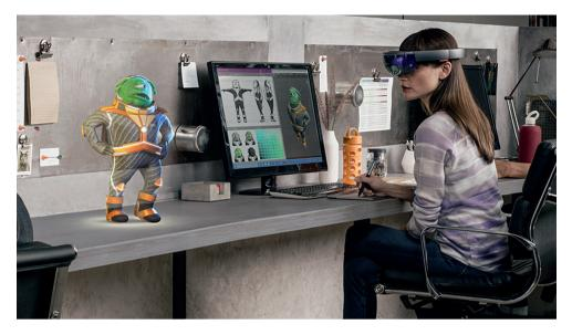
**Figure 1.20** The Microsoft Hololens, first generation, uses advanced see-through display technology to superimpose graphical images onto the ordinary physical world, as perceived by looking through the glasses.
