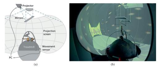
**Figure 1.2** (a) An experimental setup used by neurobiologists at LMU Munich to present visual stimuli to a gerbil while it runs on a spherical ball that acts as a treadmill [330]. (b) The gerbil appears to be in a panoramic movie theater.
