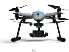
**Figure 1.12** Examples of robotic avatars. (a) The DORA robot from the University of Pennsylvania mimics the user's head motions, allowing him to look around in a remote world while maintaining a stereo view. (Panoramas are monoscopic.) (b) The PlexiDrone, a flying robot that is designed for streaming panoramic video.
