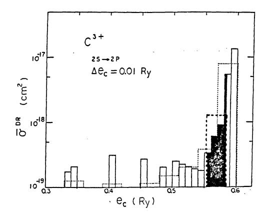
Figure 2. A theoretical dielectronic recombination cross section for  $C^{3+}$ averaged over a bin size  $\Delta e = 0.01$  Ry. The shaded section illustrates the energy averaged cross section to be expected in the present experiment (from McLaughlin and Hahn, 1983).
