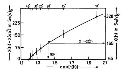
Figure 2. Elevation dependence of the atmospheric correction term X(h). To set up an absolute scale for X(h), 64 and 73  $S_{10}(V)$  were used for the brightnesses of background starlight at the north celestial pole and zodiacal light there at the time of observation, respectively.
