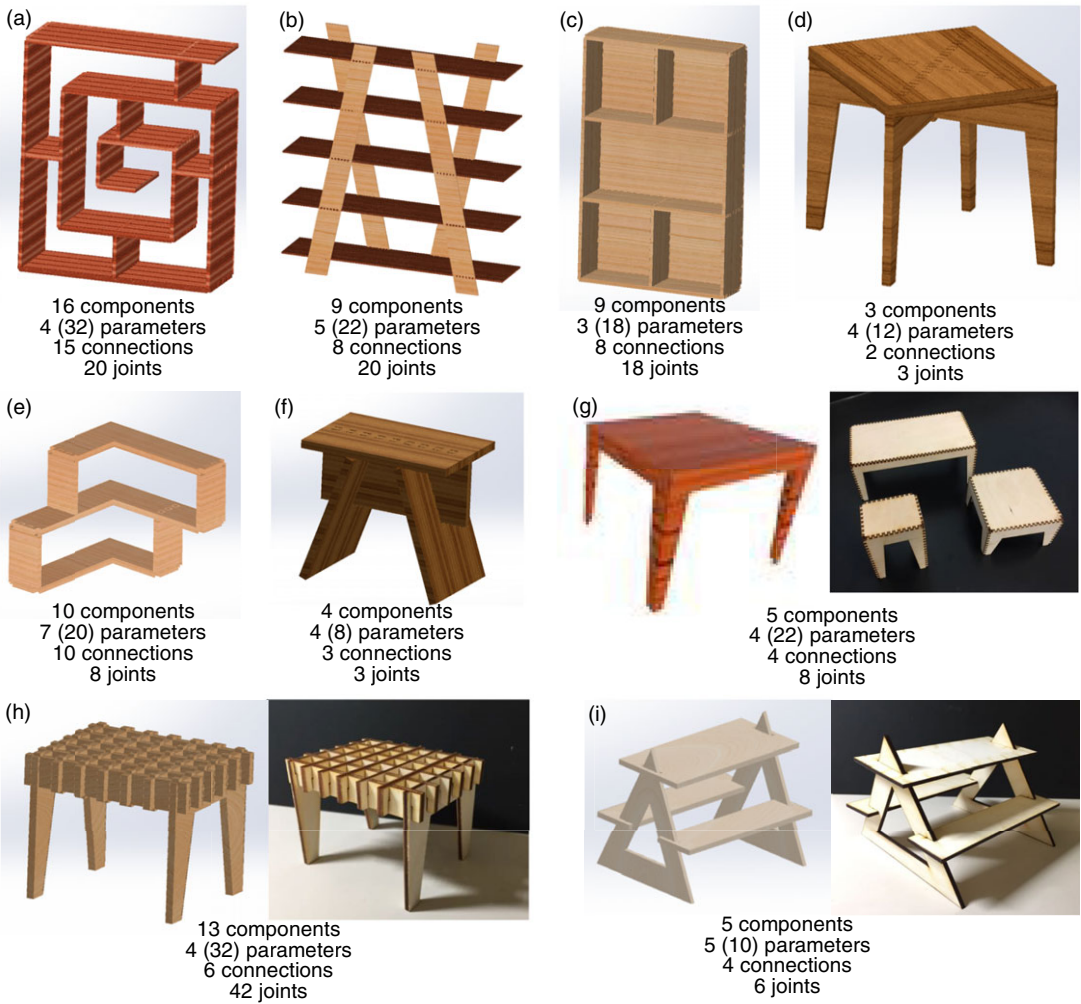
Figure 11. Furniture design examples using our system. The numbers of components, available design parameters, connections, and joints of each design are labeled. For design parameters, the structure-preserved values are calculated after some constraints are added to preserve the structure of the designs while the maximal values are included in brackets.
