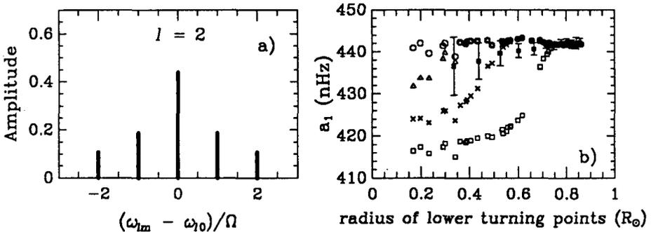
FIGURE II a) Rotational multiplets for whole-disk observations ( $\alpha = 30^\circ$ ); b) Averaged rotational splitting coefficients  $a_1$  [as defined by Duvall *et al.* (1986)] with  $(r_c/R_\odot, \beta) = 0, 0$  ( $\circ$ );  $0.3, 40^\circ$  ( $\Delta$ );  $0.5, 40^\circ$  ( $\times$ );  $0.7, 40^\circ$  ( $\square$ ) together with BBSO data (with error bars)
