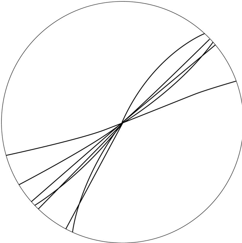
Figure 1.9 An example of an  $e^+e^-$  annihilation event that results in two jets of hadrons. The figure shows the projection of the charged particle tracks onto a plane perpendicular to the axis of the  $e^+e^-$  beams. This figure was taken from an event in the TASSO detector at PETRA DESY.
