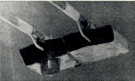
*Fig. 6. The wet and dry thermocouples at 213 cm.*
