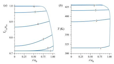
FIGURE 12. Droplet profiles as a function of normalized radius  $r/a_0$  for instants marked from 1 to 6 in figure 11. (a) The *n*-hexadecane mass fraction profiles. (b) The temperature profiles. Solid light lines show *n*-hexadecane mass fraction (a) and temperature (b) at the droplet surface r = a(t).
