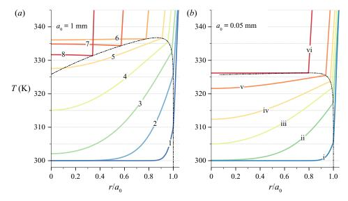
FIGURE 6. Ethanol droplet temperature profiles as a function of normalized radius  $r/a_0$  for instants marked in figure 5. (a) Temperature profiles for initial droplet radius of  $a_0 = 1$  mm at time instants 1 to 8 indicated in figure 5. (b) Temperature profiles for initial droplet radius of  $a_0 = 0.05$  mm at time instants i to vi indicated in figure 5. The dot-dashed line represents the evolution of the surface temperature  $T_s$ .
