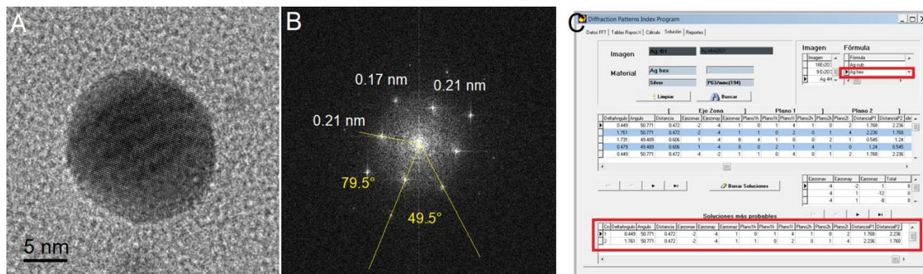
Figure 1. (A) HRTEM image of a single AgNP, and (B) its FFT. The measured interplanar distances and angles are shown. (C) A screenshot of the DPIP interface displaying the calculated interplanar distances and angles.
