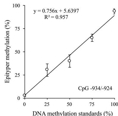
**Figure 1.** Linear association between unmethylated (0%), 35, 50, 75, and 100% methylated samples for individual and mean values across target region (cytosine phosphodiester guanine [CpG] -934/-924) in the EpiTYPER assay. Each standard was run in triplicate. The error bars are indicative of standard error.
