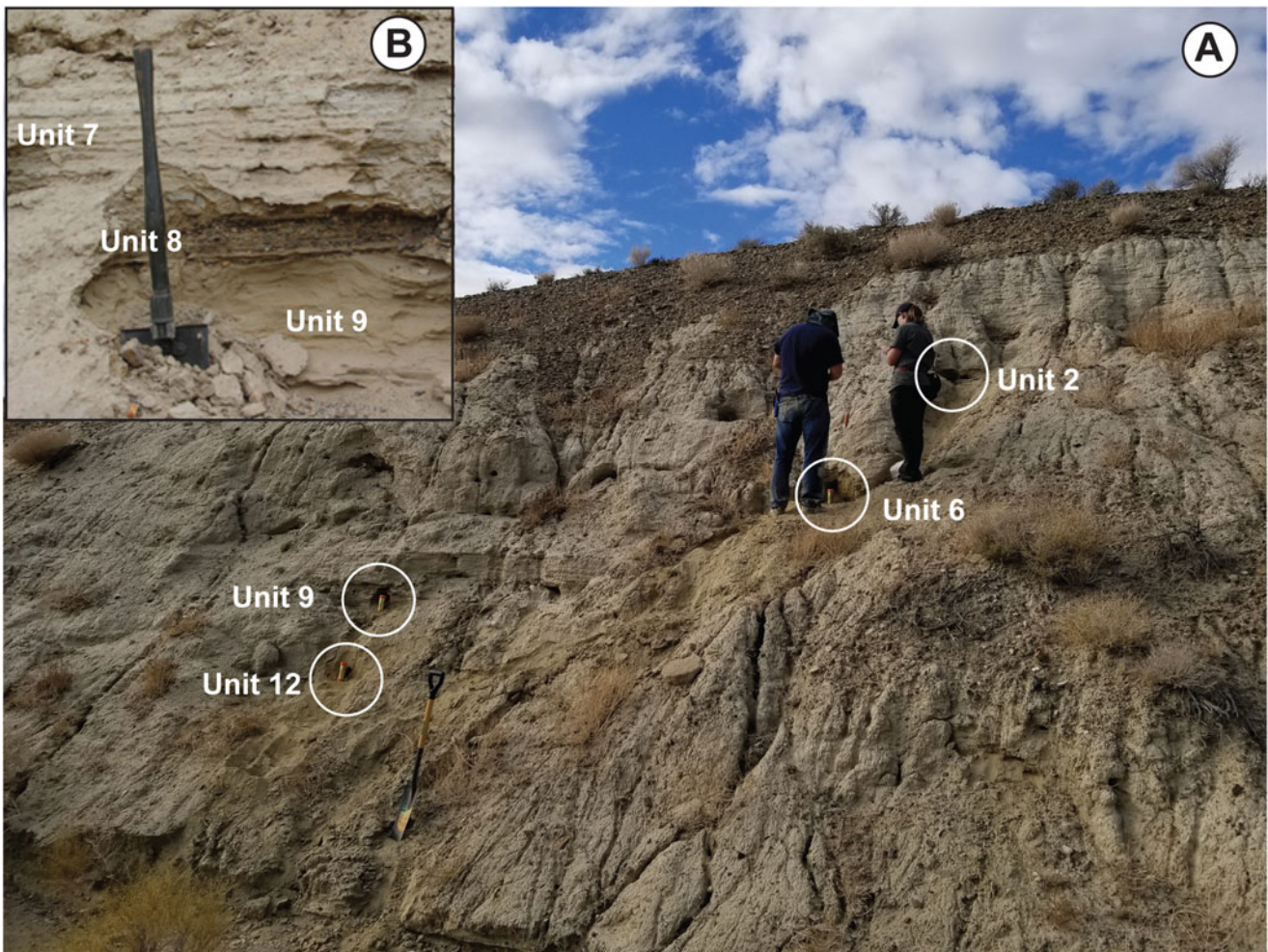
Figure 5. (A) Older lake beds of Deep Springs Valley where stratigraphic section was measured with locations of luminescence samples (circles) collected. (B) Close-up of massive sandstone of unit 9 overlain by pebbly conglomerate of unit 8 and poorly cemented mudstone of unit 7. See Figure 6 for full descriptions of units.
