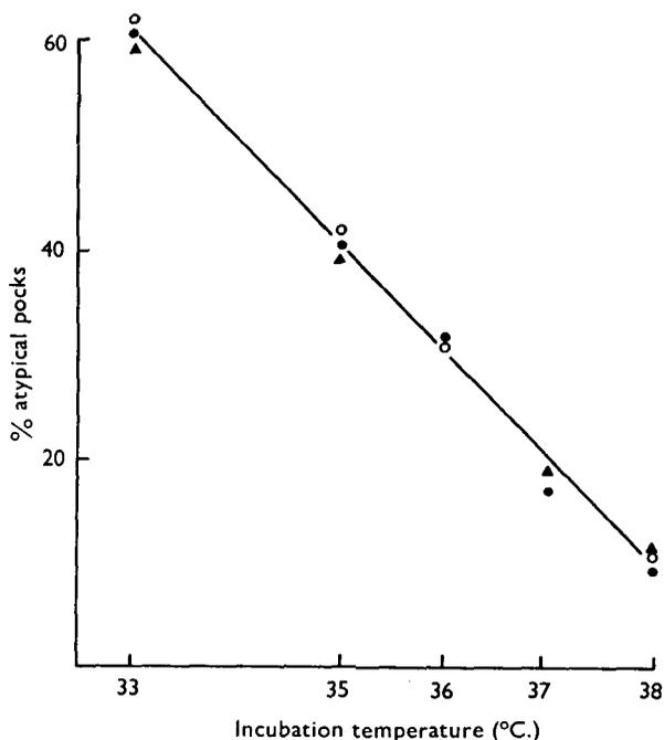
Fig. 1. Effect of incubation temperature on production of atypical pocks by white cowpox. ●, ○, ▲, three separate experiments.
