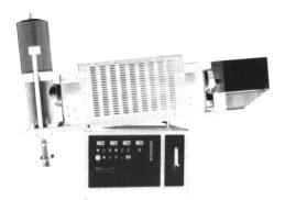
**Rotary Tubular Furnaces** for heat treatment of metallic and ceramic powders, waste and special waste, with or without protective gas, at temperatures up to 1100° C with metal tube, up to 1200° C with quartz tube, up to 1600° C with ceramic tube, up to 1900°C with sapphire tube. Variable rotary speeds, tiltable, also without post combustion or other accessories available.
