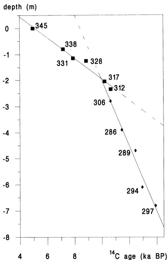
Fig. 3. Radiocarbon ages vs. depth correlation for small crystals of calcimicrite. The sedimentation rate is  $0.25 \text{ m ka}^{-1}$  for carbonate dominated sediments (■), compared with  $1.25 \text{ m ka}^{-1}$  for gypsum dominated sediments (◆). The lower sedimentation rate corresponds to the last lacustrine episode (4–10 ka BP), for which the catchment supply was more significant. The gypsum-dominated sedimentation prior to 10 ka BP corresponds to more arid conditions.
