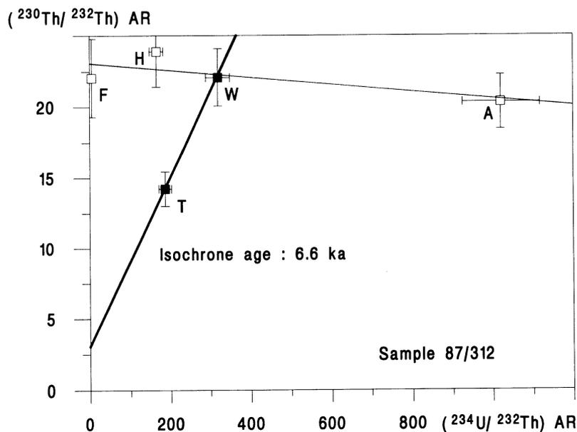
Fig. 4.  $(^{230}\text{Th}/^{232}\text{Th})$  AR vs.  $(^{234}\text{U}/^{232}\text{Th})$  AR correlation diagram for Sample 87/312. A – acetic acid leachate; H – HCl leachate; F – totally dissolved residue; W – for the whole sample reconstructed from leachate data; T – a separate sample, totally dissolved.
