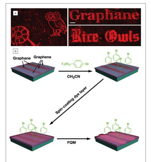
(a) Images of graphane/graphene patterns revealed with fluorescence quenching microscopy (FQM); the scale bars are 200 μm; (b) the fabrication of sp³ C–C exchanged superlattices and subsequent FQM imaging is illustrated with a schematic diagram. Reproduced with permission from *Nat. Commun.* **2**:527, DOI: 10.1038/ncomms1531. © 2011 Macmillan Publishers Ltd.
