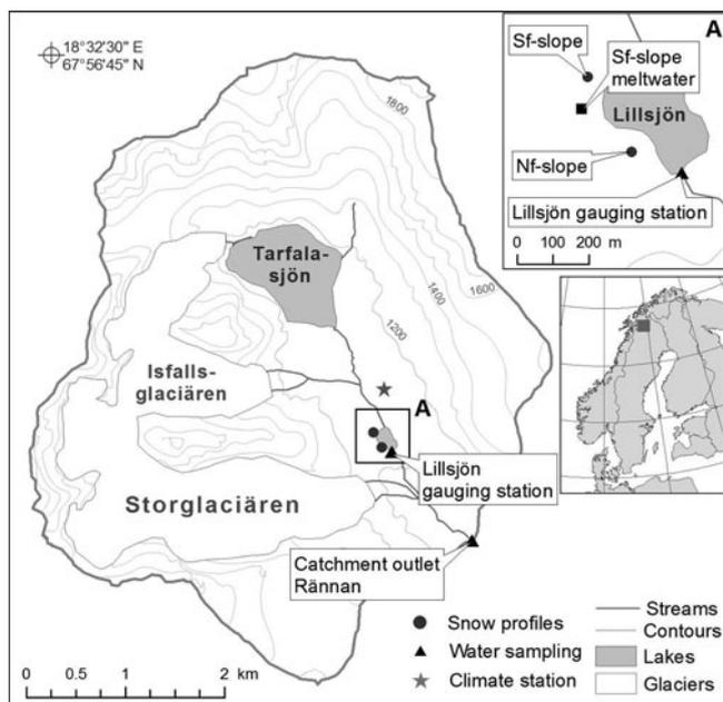
**Fig. 1.** Location of the Tarfala research catchment in northern Sweden, the climate station (near Tarfala research station), gauging stations (Lillsjön and Rännan), snow profiles (Sf and Nf slope) and meltwater sampling sites (Sf slope meltwater).
